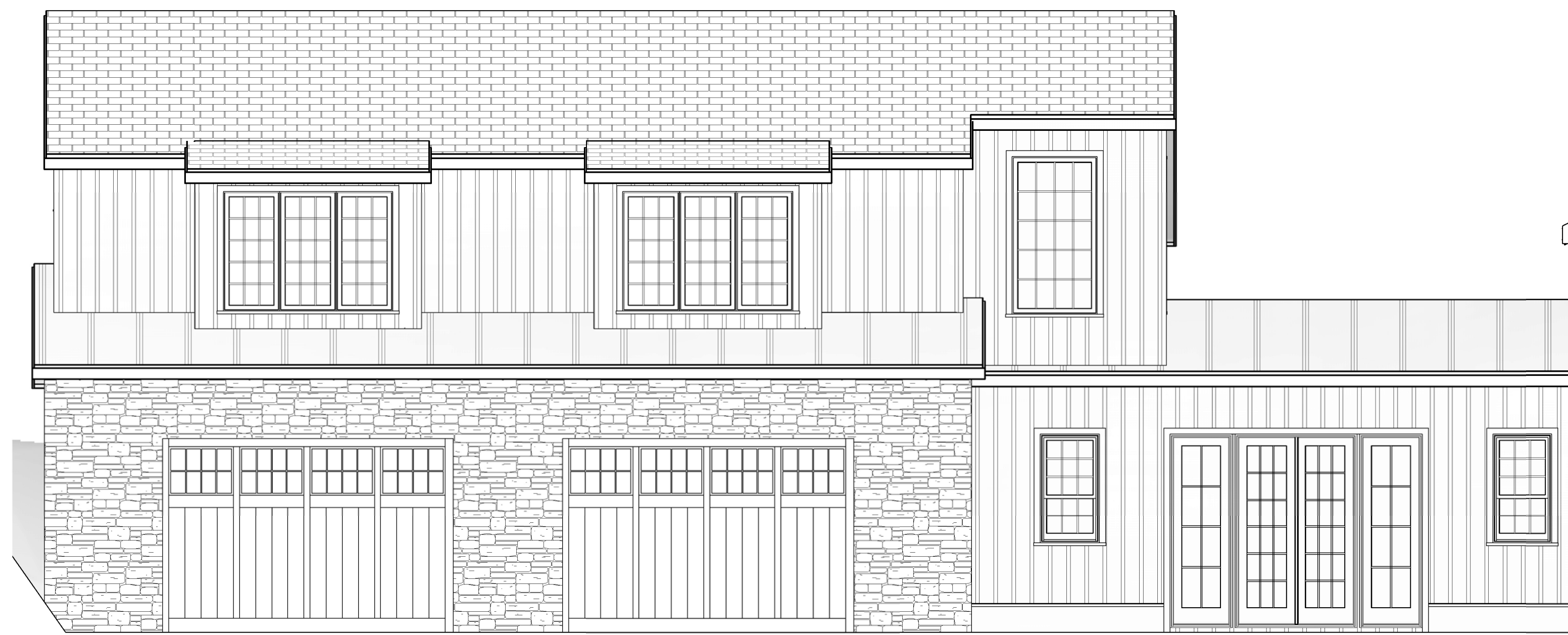
4 GARAGE/SCREEN PORCH NORTH ELEVATION A2.1 1/4" = 1'-0"
