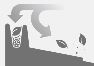
Dirt gets stuck in other double-hung window sills
