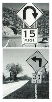
The advisory speed must be determined by an accepted traffic engineering procedure but no ordinance is required. Maintenance or sign supervisors can erect the signs. They must be in accordance with guidelines in the *MUTCD*, 2C-35.
